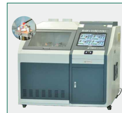
热电偶耐久测试仪 Thermocouple Endurance Tester
